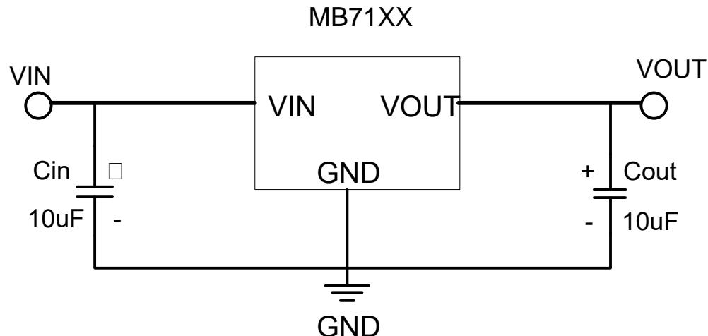
Note1:  $C_{in}=C_{out}=10\mu F$ . (10 $\mu F$  Electrolytic capacitor is recommended).
