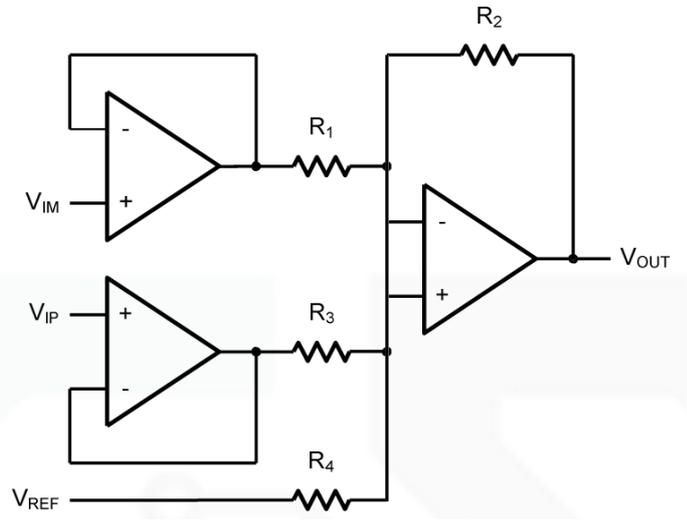
Figure 6. Instrument Amplifier
