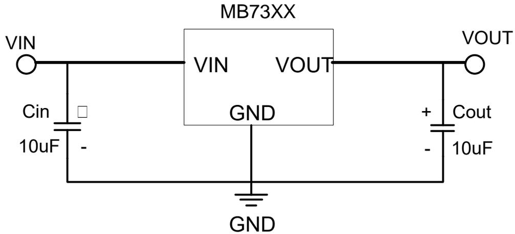
Note1:  $C_{in}=C_{out}=10\mu F$ . (10 $\mu F$  Electrolytic capacitor is recommended).
